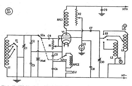
Fig. 1. The VFO-CO unit described by G3XT. It can be operated as a low-power transmitter as it stands and has performed well as such.
