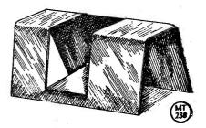
Fig. 2. The chassis bend suggested by G3XT to produce the finished effect shown in the photograph.
