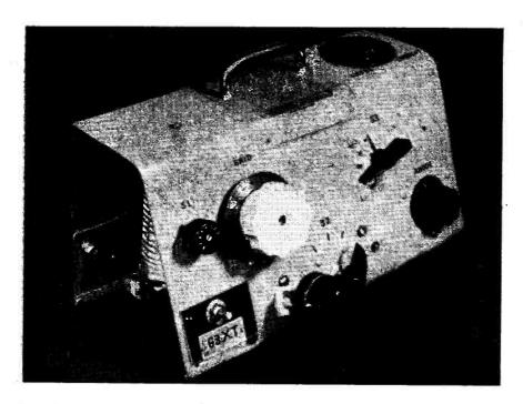
General appearance of the single-valve oscillator as constructed by G3XT. It can be keyed direct for QRP working.
