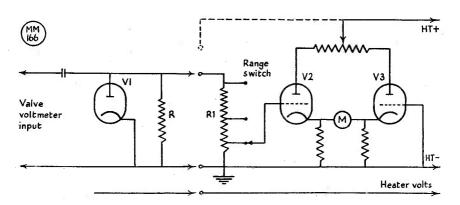
Fig. 1A. A valve voltmeter with external diode probe; this can be inter-changeable with a GDO to use the same meter and power supply—see Fig. 1B.
