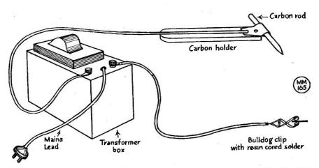
Sketch showing general arrangement of the LT soldering method suggested by G6AB in his article
