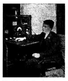
GSUN of Prestwich, Manchester, believes in taking his radio in comfort. Though licensed since 1938, he has never gone QRO and the main interest still is phone on Twenty with 10 watts to an 807. The Tx is VFO controlled, the aerial a folded dipole fed with 300-ohm ribbon, and the whole outfit is relay controlled. And when the top and two lower doors of the operating desk are closed, none of the gear is visible—an ideal living-room layout.
