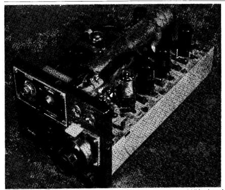
General view of the ASB8 after modification, showing the front panel controls. Additional panel bracing struts (not shown) should be fitted to provide better mechanical stability for the 1st oscillator.
