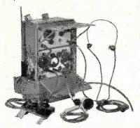
The "48" has a frequency range of 6-9 mc/s (33.3-50 M.) and comprises a transmitter equipped for 'FON or CW operation, VFO control, driving a pair of 1299's in the final at an approximate input of 8 watts, and features a built-in modulator and a 1,000 kc/s freq. standard complete with crystal, and a "netting" device which allows the transmitter to be VFO'd spot on to any signal received without the Tx final being operated. A morse key and microphone is supplied.
