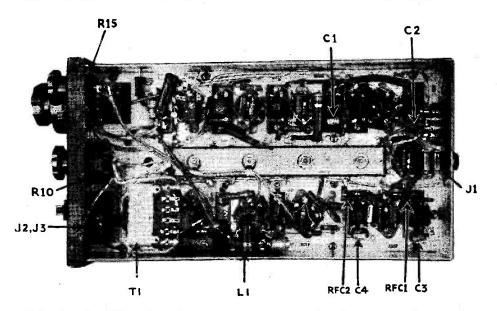
Underside of the ASB8, with positions of major new components indicated. As in the original every circuit element is numbered and the under-chassis layout is particularly clean, there is no difficulty in finding one's way about it.
