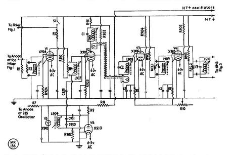
Fig. 2. The IF section of the ASB8 after modification. The original component numbering is used for ease of identification, new circuit elements only being designated in the C, R, L nomenclature.
