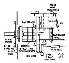
Fig. 4. Modifications suggested to 1st oscillator stage to enable condenser tuning to be used.
