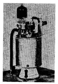
The 430 mc pot oscillator now in use at G&VR. Valve is a 9002, the copper (petrol) pipe on the left takes the live heater lead to the valve and acts as cathode return, and the two resistors visible are anode decoupling and grid leak. The inner can is from a CV173 and the outer is an old valve screen. Stability is excellent and output coupling is by means of a hairpin loop in a hole drilled into the pots.
