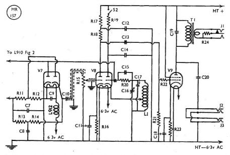
Fig. 3. Detector, noise limiter, BFO and audio stages as applied to the ASB8 to make it a receiver complete in itself.
