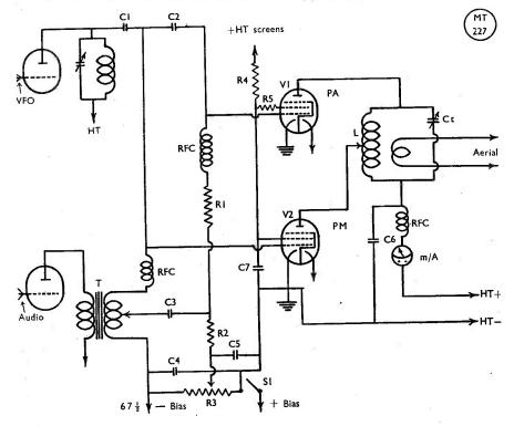
Fig. 4. Circuit used for ORP battery-operated transmission, applying Super Modulation. G2BCX has tested this arrangement on the Top Band, and the table gives values for 160-metre working.
