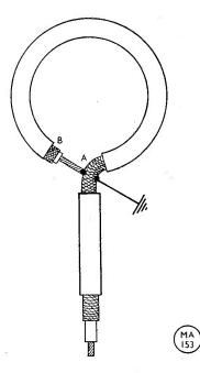
Fig. 3. Suitable screened coupling loop constructed from a length of coax, as described in the text.
