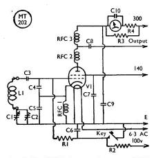
Circuit of the 807 VFO driver unit described by G3BTP. By the use of two coils, for 1.7 and 7 mc, at L1, stable output is obtainable on all bands 1.7-28 mc to drive a following 807 to 25 watts.
