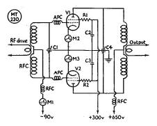
Fig. 2. Basic circuit to which Super Modulation can be applied by the modifications shown in Fig. 3. As explained in the article it is better to get this circuit working correctly before attempting the modification and the anti-parasitic chokes APC are essential.
