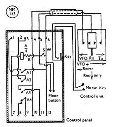
Fig. 1. General arrangement of the switching and control system devised by G2QY and discussed in the text. The key for the connections is given separately.
