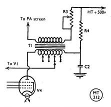
Fig. 2. The 6V6 modulator and modulation transformer as shown here illustrate the method of tapping the HT feed for V1 towards the anode of V4, thus previding a greater audio swing at the control grids of V2, V3.
