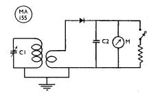
Fig. 5. A simple RF detector for investigation of current distribution along feeder and aerial systems, as discussed in the article. C1, C2 are 0001  $\mu$ F and M is 0-1 mA
