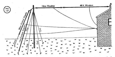
Fig. 1. Having noticed how coats can be hung round a hat-stand, GSUA decided to use his mast as a suspension fer vertical aerials, somewhat in the manner shown in the aketch. His system consists actually of four separate aerials two vertical, and two horizontal. Vertical or near-vertical aerials have the great advantage, on the HF bands, of almost omni-directional radiation.
