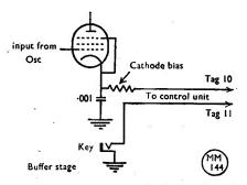
Fig. 2. The VFO connections in the control circuit.
