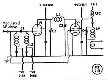
Fig. 1. If the effective load of L4, C4 with aerial connected is R1 ohms, then  $\omega L3 = 2R$ ;  $1/\omega C2 = 2R$ ; and  $1/\omega C3 = 2R$ . If the grid input resistance of V1 is R2 ohms, then  $\omega L1 = R2$ ;  $\omega L2 = R2$ ; and  $1/\omega C1 = R2$ . There should be no mutual inductance between L1 = M2. L1 and L2.
