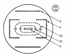
Fig. 1. Electrode arrangement of a transit-time controlled oscillator valve.
