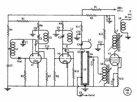
Fig. 2. Circuit complete of the 70 cm, converter designed and described by G3EJL. All values appear in the table.
