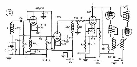
Fig. 1. From the CAY-47155C, G3BYV produced this circuit arrangement, the result being a useful Top Band transmitter.
