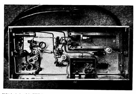
Under-chassis view of the G3EJL 70 cm. converter showing general arrangement and, top right, the Lecher tuning section of which full details are given in the text.
