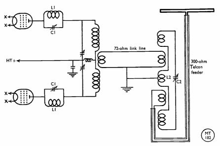
Fig. 2. Circuit arrangement of the aerial coupling network. The links on L2 are spaced equidistant from the earth tap. L1, 8 turns No. 16 SWG,  $\frac{3}{2}$  in.i.d., 1 in. long; L2, 10 turns overall,  $\frac{1}{2}$  in. dia. copper tube,  $2\frac{1}{2}$  in.i.d.; C1, 3-30  $\mu\mu$ F trimmers; C2, 50  $\mu\mu$ F, spaced for voltage. These values are for 14 mc operation.
