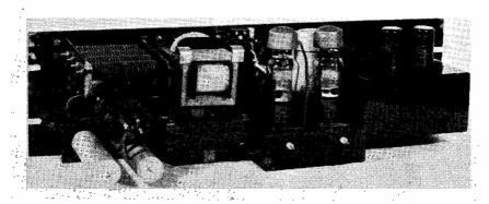
Rear view of the VFO section of G2QY's transmitter, with the oscillator unit itself at the right, and the amplifier-doubler chassis at centre. All details are given in the text.
