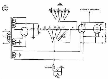
Fig. 5. The valve keyer suggested by G6HL; the current capacity can be increased by paralleling further valves with V1, V2. Values are given below and the method of operation is covered in the discussion.
