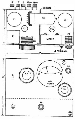
Fig. 2. Suggested chassis layout for the G5RZ QRP design, giving dimensions and essential layout details.
