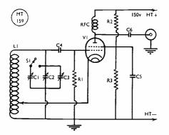
Fig. 1. The VFO driver circuit suggested by G2NS. Functions of S1 and C1-C3 are explained in the text.
