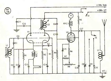
Fig. 1. The 1.7/3.5 mc QRP transmitter unit described by G5RZ, discussed in the text and illustrated in the photographs.
