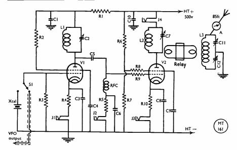
Fig. 3. Circuit complete of the VFO/CO-PA transmitter for the Top Band, discussed in the article.
