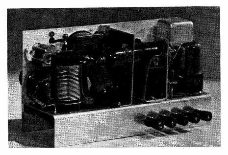
Rear view of the G5RZ QRP job, showing general arrangement of the parts and mounting of the valves.
