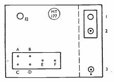
Fig. 2. Rear view of the CAY-47155C chassis, showing socket connections.
