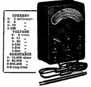
A conveniently compact 2½-inch moving coil precision meter for making D.C. measurements of milliamps, volts and ohms. The total resistance of the meter is 100,000 ohms, and full scale deflection of 300 v. or 600 v. is obtained for a current consumption of 3mA. or 6mA. respectively.
