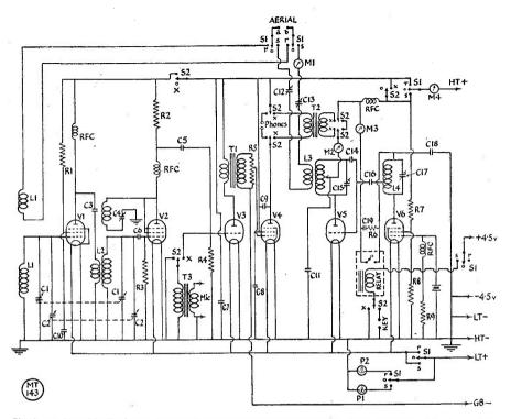
Circuit complete of the CW/<sup>2</sup>phone portable 40-metre station designed by G3ECX. Valves V1-V4 comprise the receiver section ; V6 is the CO-driver and V5 the PA on the transmitting side. For 'pnone operation, V3-V4 become speech amolifier-modulator. The photographs suggest how this circuit can be built up as one compact unit, entirely self-contained.
