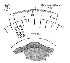
Fig. 2. Calibration card fixed to the main dial.
