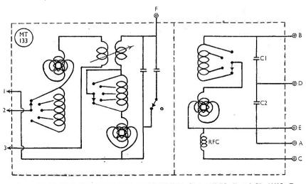
Fig. 1. Circuit of the tuning section of the CAY-47155 Unit. C1 is 000625  $\mu$ F, and C2 00125  $\mu$ F.
