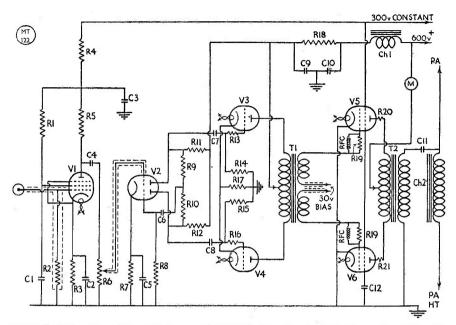
Full circuit of the speech amplifier-modulator operated by G5NH. Saturation of the modulating transformer is avoided by the parallel feed connection shown at the output end. Though it does involve an additional heavy component, in fact any good choke capable of carrying the PA plate current will suffice—and there is often one such spare at most stations.
