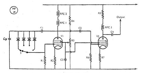
Fig. 2. Another version of Fig. 1, using 6SH7's for V1 and V2. Values are given in the table.
