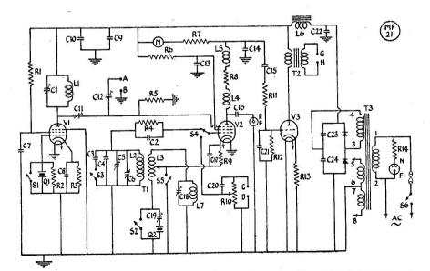
Fig. 2. Circuit diagram of the Wide-Range Heterodyne Frequency Meter, simplified as to switching (see Fig. 3.) It is an instrument having many useful practical applications in any amateur statuon and can be built from standard parts.
