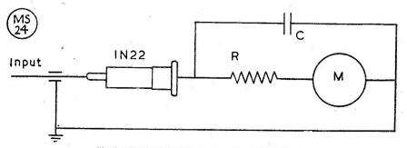
Fig. 3. Circuit of the HF voltmeter. described in the text.
