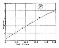
Fig. 1. G2NX's method of obtaining interpolated readings from the main calibration curve.
