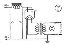
Fig. 5. An arrangement for obtaining bias voltages for a high power transmitter.
