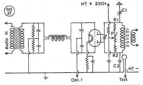
Fig. 6. Some desirable modifications to the balanced modulator stage. R1, R2, 3,000 ohms, ½-watt ; P1, 750-ohm w/w potentiometer ; C1, 50 μμF variable, ceramic ; C2, 25 μμF ceramic. All other values are as given for Fig. 17 p. 428, August issue Short Wave Magazine.
