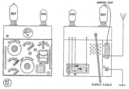
Fig. 4. Sketches suggesting front and rear views of the completed conversion, based on the CAY-47155 foundation.
