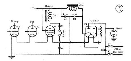
Fig. 2. The author suggests this as an improvement on the rectifier arrangement shown in Fig. 1.
