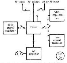
Fig. 1. Block schematic showing the electrical interconnection of the units in the instrument, and the functions it can perform.
