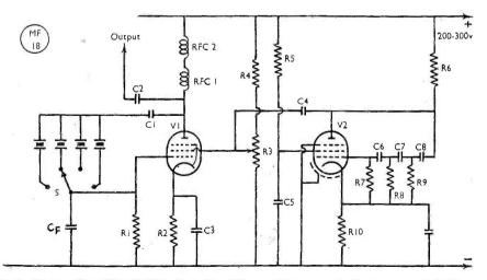
Fig. 1. Pierce oscillator (V1) with RC audio oscillator (V2) to modulate the signal. Good output is obtainable over a wide range of harmonic frequencies.
