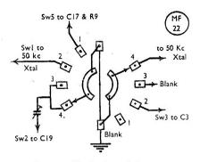
Fig. 3. Diagram showing the switch connections, as devised by the author to produce the changes shown in Fig. 1.
