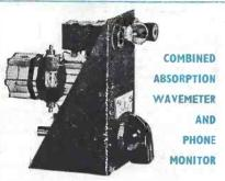
An Absorption Wavemeter for checking har-monics and parasitics; and oscillators, doublers and power amplifiers for correct frequencies. All amateur bands are covered by means of plugin inductances.
