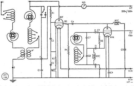
Fig. 5. The circuit complete of G2CZ's Top Band transmitter, as described in the article. In this diagram, C7, C8, are the C1, C2, of Fig. 1.
