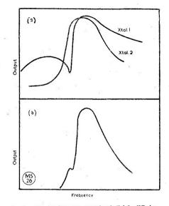
Fig. 5. Showing how two crystals of slightly differing frequencies (a) may be combined as in (b) to produce a steep-sided response suitable for an SSB filter.
