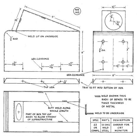
Fig. 2. For those who would like to make it neat and tidy, here are the detail drawings for the fabrication of the metal cabinet to house the unit.
