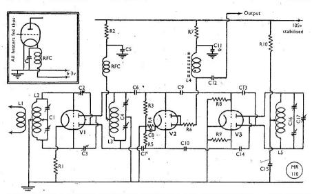
The circuit complete of G2IQ's two-metre converter, using 6J6's and with a neutralised RF section. It is a low-noise high-gain iob, easy to build, and should give exceptional results on Two. The by-pass condenser C in the sketch inset can be 500  $\mu\mu$ F.
