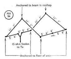
Physical layout of the indoor aerial system for 7 mc, devised by G3BQJ.
