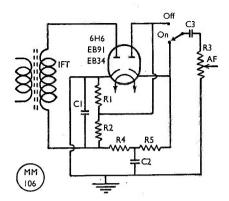
Circuit incorporating G2AKY's ideas for an effective noise limiter; details are given in the text.
