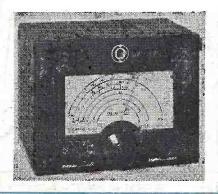
This is a V.F.O. employing the series tuned Colpitts (Clapp) circuit, and is extremely stable and free from drift. Output at 3.5; 5.25 or 7 Mc/s. Calibration on all, amateur bands from 3.5 to 30 Mc/s. High or low impedance output to drive voltage or power stages.
