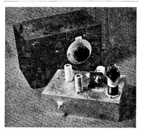
The second (and more "decent") converter referred to in the text. This is built up on an Eddystone chassis and incorporates a voltage regulator.
