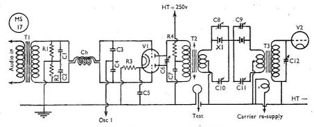
Fig. 17. Circuit of the balanced modulator-see text for discussion.
