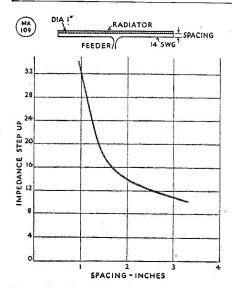
Fig. 3. Design data for folded dipole used as a radiator. As an example, for 12-in. spacing between tube and wire the feeder impedance divided by the radiator impedance is 18, representing an impedance step-up of 18 times over a plain dipole in the same position.
