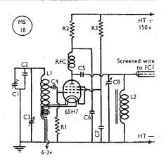
Fig. 18. ECO circu t for Osc. 2, covering 1.8-2.2 mc. Any suitable oscillator can be employed for this position
