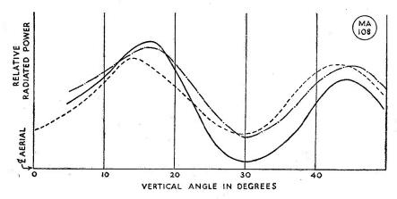
Fig. 2. Showing power distribution pattern (vertical plane in forward direction) for beam arrays adjusted as follows: 3-ele. close-spaced, maximum front-to-back ratio, dotted line; 3-ele. close-spaced, maximum forward gain, chain dotted; 4-ele. close-spaced, adjusted for maximum forward gain, solid line. In each case the height above ground is one wavelength and the element spacing 0·1 wavelength.
