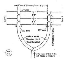
GW3ZV suggests this "Three-by-Three" for 145 mc. All elements are 39-in. of ½-in. tubing, stacked 39-in. A single bay could be used separately and fed by 600-ohm open line. Note the transposition points, also using open wire line and with connections between elements kept as short as possible. The array as dimensioned is two-way looking, giving a clover-leaf pattern broadside to the plan of the elements, and the lobes are approximat ly 60 deg. wide at half-power points.
