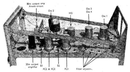
Showing general layout of G2NX's SSB Driver, in the early stages of construction on an adapted R.3170 chassis. The Schematic at Fig. 10 keys this photograph
