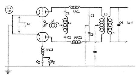
Fig. 8. A grounded-grid triode converter stage, some points regarding which are covered in the article.
