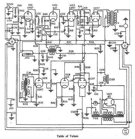
Fig. 2. Circuit diagram of the BC-614 Speech Amplifier, which can be modified quite easily for amateur operation, as described in the text.
