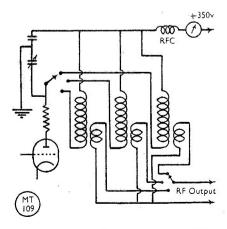
Fig. 4. Switching at the output end of the G4QK Exciter.
