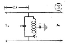
Fig. 2. Using part of the aerial feeder line as a blocking filter for the unwanted asymmetric voltage.
