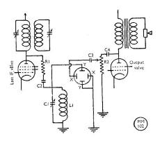
Connecting a cathode-ray tube into the receiver for observing the characteristics of an incoming signal; G8LO explains this circuit in the accompanying text.
