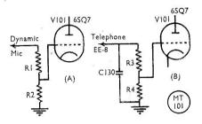
Fig. 1. Equivalent input circuits of the microphone matching system in the BC-614. The resistor values are: R1, 536,000 ohms; R2, 9,000 ohms; R3, 1,000 ohms and R4, 100 ohms
