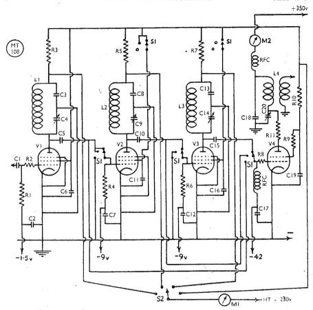
Fig. 3. Circuit of the G4QK Exciter complete. EF50's are used in the oscillator-doubler stages, with an 807 as output driver; the circuits are arranged to give level excitation, without re-tuning, over each band.
