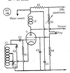
This article describes an efficient broad-band exciter, the design of which is of particular interest. The oscillator-doubler stages use the popular EF50, with an 807 as final buffer-doubler, making altogether a flexible unit which is cheap, easy to build and capable of excellent results.-Ed.
