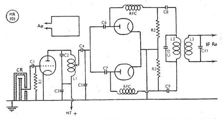
Fig. 5. Complete practical circuit for a diode converter stage, using a cavity resonator (CR in the diagram) in the grid of the oscillator, an arrangement very suitable for frequencies around 300 mc.
