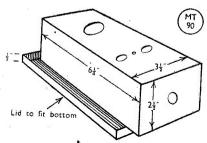
Fig. 2. Dimensions of the chassis-screening box, as actually used; they can be varied to suit individual requirements.
