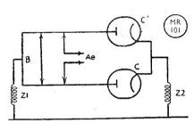
Fig. 3. A variation on Fig. 2., where the aerial feeder connection is taken to points on the input circuit having minimum asymmetric voltage.
