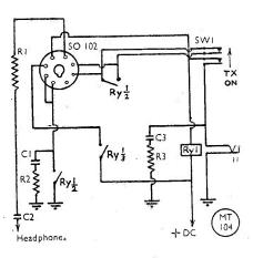
Fig. 4A. The BC-614 control circuit.
