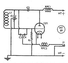
Fig. 1. Circuit of the oscillator unit suggested by G3XT.
