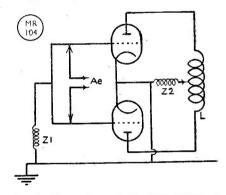
Fig. 6. Circuit for a push-pull triode converter, as discussed in the text.
