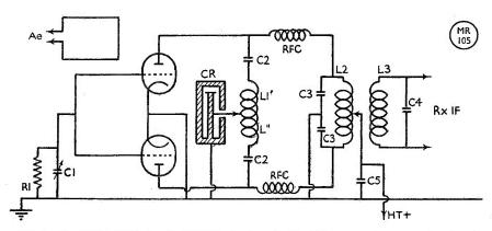
Fig. 7. Complete circuit diagram for a triode converter, using a cavity resonator for frequency stability
