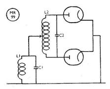
Fig. 1. Two diodes connected to an asymmetric circuit L1/C1 and a push-pull circuit L2/C2.
