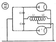
Fig. 4. A basic converter circuit with Lecher wire input, free of asymmetric voltage.
