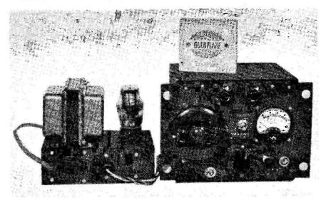
The transmitter and associated power supply. That (empty) Gold Flake packet well suggests the very small size of the two units.
