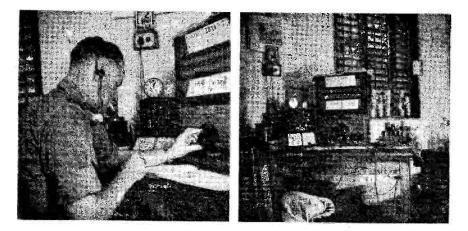
The outfit (and operator) at VS7PH, Negombo, Ceylon. The Tx is 6L6-807, 25 watts, into a 14-mc dipole, with an Australian-built receiver. On this rig VS7PH (who is GAATH of Skipton, Yorks) has had 1,000 QSO's with 94 countries in 38 Zones.
