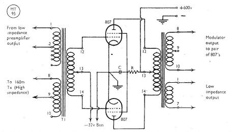
Modulator used by G2QY, utilising for T1 and T2 transformers from the Type 51/APQ9 power pack; in this circuit C is 2  $\mu$ F and R 35,000 ohms. Voltage ratios of the transformers are shown in the accompanying table.
