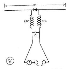
Fig. 1. The basic arrangement, but unsuitable without the modifications discussed in the text. C is  $\cdot 0001 \ \mu F$ .
