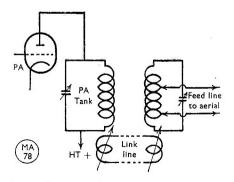
Fig.<sup>\*</sup>2. Coupling the PA to the aerial tuning circuit proper, through a long feeder line—see text for detailed discussion.
