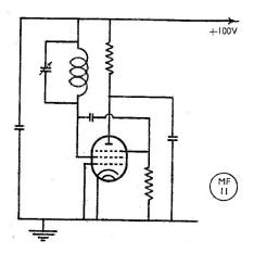
Fig. 2. The Transitron oscillator; the theory of operation of this circuit was discussed in our issue for June 1947.
