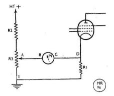
Circuit suggested for S-meter connection to an existing receiver, as described in the text.
