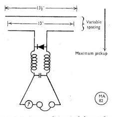
Fig. 4. Putting on a reflector not only increases the pick-up in the desired direction, but also enables the impedance appearing at the crystal to be varied.
