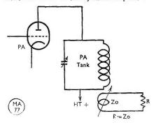
Fig. 1. Resistance R is equal to the characteristic impedance (Zo) of the transmission line.
