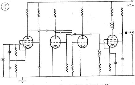
Fig. 1. Conventional crystal oscillator, multivibrator and harmonic amplifier.
