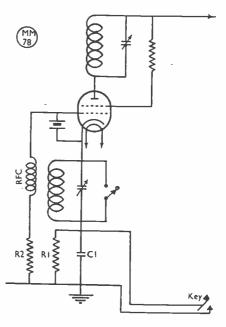
GM8RV's keying circuit; R1 is 10,000 ohms, and C1  $02 \mu F$ . It involves a small standing current on the valve to produce a self-biasing voltage.
