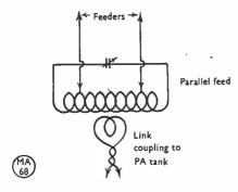
Fig. 6. Parallel tuned feeder connection.
