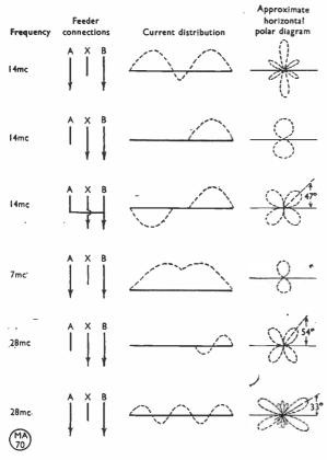
Fig. 8. The current distribution for different feeder connections from band to band, showing also the approximate radiation pattern under different conditions.
