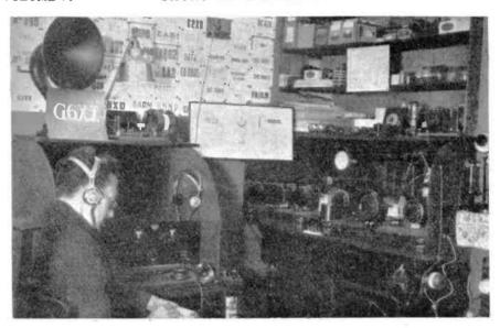
Early in 1929, G6XJ (now a director of Stratton & Co., Ltd., manufacturers of Eddystone equipment) operated this station in Birmingham. Two TPTG transmitters were run off the DC mains boosted by HT accumulators, and the receiver was a 1-V-1. Time marches on!
