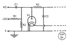
Fig. 3. The diode probe, described in the text.
