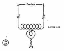
Fig. 7. Series tuned feeders.
