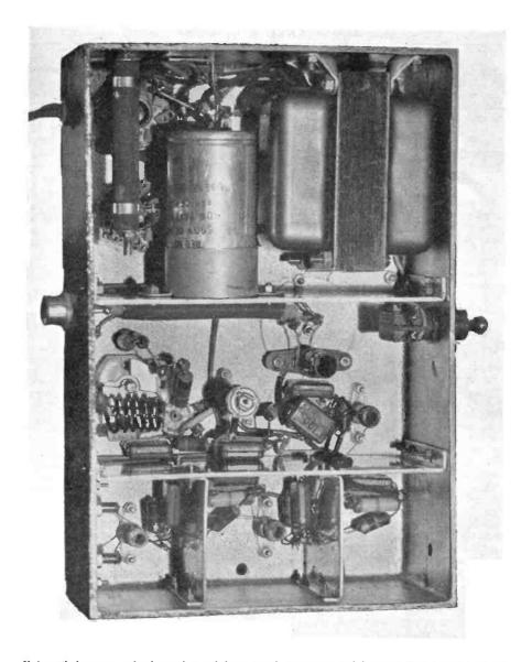
Underneath the converter chassis; each stage is in a screened compartment, and the overall dimensions of the chassis are only 8½-in. × 6-in. × 2½-in. deep. Miniaturised components are used throughout, including the Smith smoothing choke (top right) in the power compartment.
