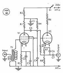
Fig. 1. Circuit of the pre-amplifier.
