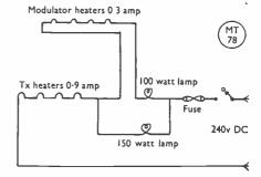
Fig. 3. Connections for the heaters on transmitter and modulator, fed direct from the DC mains. The lamps are taken out on wandering leads, and the power they dissipate as series resistors lights the station!
