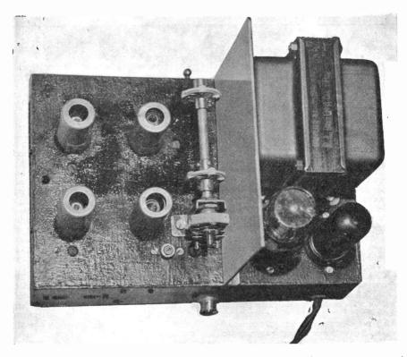
The RF, mixer and oscillator valves are in sprung screening cans and with the oscillator tuning condenser are separated from the power unit by a vertical screen.
