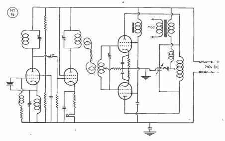
Fig. 1. Circuit for a 3-stage transmitter operated off DC mains for both HT and LT. Values would be as normally employed for the bands required. The main earth connection must be through a large condenser (2  $\mu$ F or more) rated over the working voltage.
