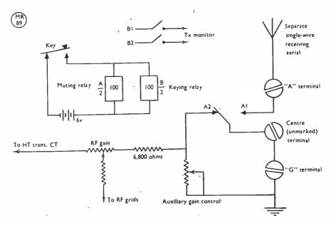
Circuit of the arrangement devised by G2NS to obtain break-in operation and full receiver protection with the AR88.
