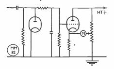
Fig. 1. Basic circuit of the valve voltmeter.
