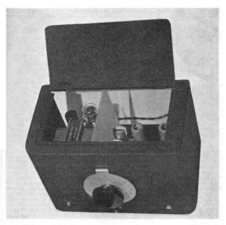
The self-powered 145-mc converter complete, in its Eddystone cabinet; the dial is the same makers' 637, with vernier, having a 10-1 reduction ratio.
