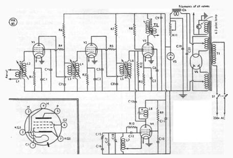
Fig. 1. Circuit of the 145 mc converter; the RF stages are broad-band so that the oscillator circuit only is tuned.
