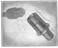
The "Belling-Lee" suppressor L630 screws into the central hole of distributor caps after removal of the H.T. lead terminal, which is then screwed into the top of the suppressor.
