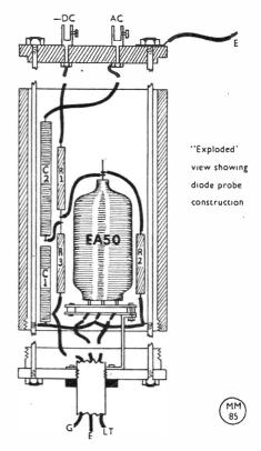
Fig. 4. Construction of the diode probe-see text.
