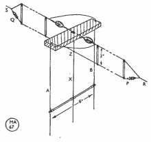
Fig. 5. Construction of the centre section of the aerial—compare with Fig. 3.
