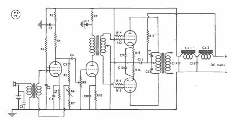
Fig. 2. DC-mains operated speech amplifier and modulator.
