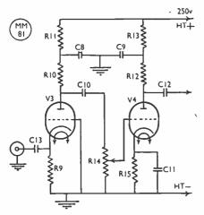
Fig. 2. Circuit for the input stage of the main modulator.
