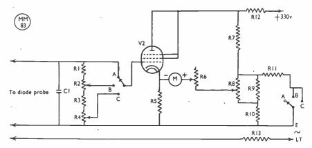
Fig. 2. Working circuit for a valve voltmeter: values are given in the table.
