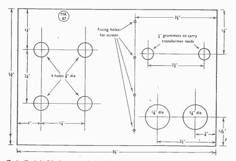
Fig. 3. Chassis detail for the converter; in the original, a standard Eddystone die-cast aluminium chassis was used (see photographs).
