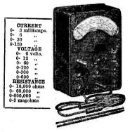
A conveniently compact 2½-inch moving coil precision meter for making D.C. measurements of milliamps, volts and ohms. The total resistance of the meter is 100,000 ohms, and full scale deflection of 300 v. or 600 v. is obtained for a current consumption of 3mA. or 6mA. respectively.
