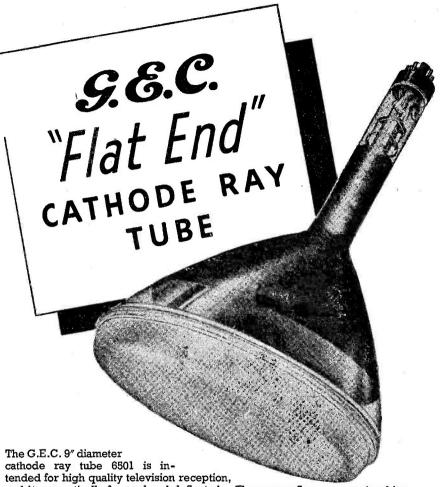
and is magnetically focused and deflected. The screen fluorescence is white.
