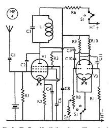
Fig. 2. The Type 18 with the audio amplifier replaced by a 6SN7 connected as a multivibrator to give the 10 kc check points.
