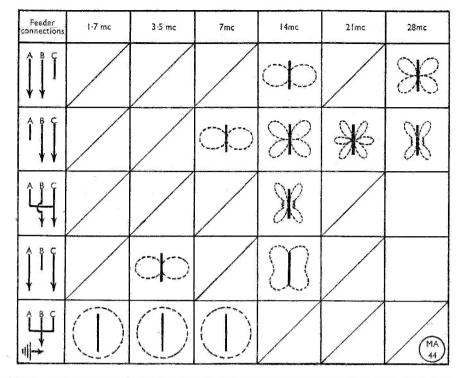
Fig. 3. (A) Radiation pattern in the horizontal plane for different feeder connections to the aerial shown at Fig. 3 (B)
