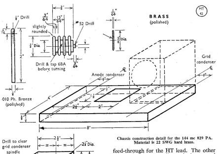
feed-through for the HT lead. The other two bushes have small terminals sweated to them to act as supports for the aerial coupling loop and aerial feeder.
