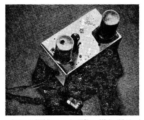
General impression of G2IQ's 144-mc converter, using a GGT RF stage, and fully discussed in the text.
