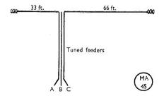
Fig. 3. (B) Dimensions for a suitable multi-band aerial, the design of which is discussed in the text.
