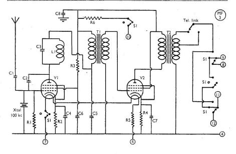
Fig. 1. Circuit of the Type 18, unmodified. The table of values applies to both Figs. 1 and 2.
