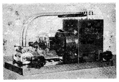
The 144 mc PA using an 829B, designed and constructed by G6VX. One neutralising wire can be seen protruding from the screening box for the input end of the amplifier. This is an RF stage which can be pushed to 120 watts on 2 metres by the exciter unit already described.
