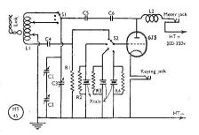
Circuit of G3XT's transmitter, discussed in detail in the text. Either CC or SE operation is possible, with a selection of crystal frequencies.
