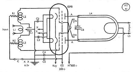
Circuit of G6VX's 829 PA for 144 mc operation. When driven by the exciter unit described in our July issue Fig. 1. it can be loaded to 120 watts input at 600 volts on the plates, and lights a 100-watt lamp to full brilliancy.
