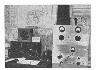
G3AWP, Winton, Bournemouth, has a BC-342 Rx, with a 6V6-807-P/P 807 transmitter operated at up to 90 watts input, using three switched crystals. Activity is on 14 mc mainly.
