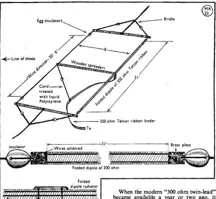
Twine bindings Third wire taped along length of dipole (see text) Method of construction of feedline joint at centre of " ribbon " folded dipole
