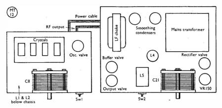
Fig. 3. Block diagram of the general chassis layout. That part of the circuit enclosed within dotted lines in Fig. 1 is in the section on the left in this drawing.
