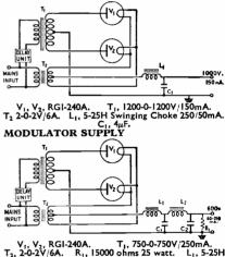
T<sub>2</sub>, 20-2V/6A. R<sub>11</sub>, 15000 ohms 25 watt. L<sub>1</sub>, 5-25H Swinging Choke 250/50mA. L<sub>2</sub>, 20H/250mA. C<sub>1</sub>, C<sub>2</sub>, 4 $\mu$ F. Write for technical data on these and other Mullard
