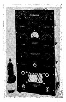
Front panel view of the transmitter, with an 807 for comparative size. The panels, from the bottom up, are : Power supply ; drive stages ; PA stage ; and aerial coupling\_unit.
