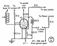
Fig. 1. Circuit of the PA side, showing how modulation can be applied. R12, 500 ohms; R13, 200 ohms, bias; R14, 1-2 megohms; C11a, C11e, C19, C20, all  $\cdot$ 002 µF; V2, 61.6. Key sockets must be shorted on "transmit" and open on "receive."
