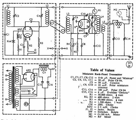
Circuit of the transmitter complete. By using twin-triodes, a CO-FD-PA arrangement can be achieved with only two RF valves.
