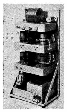
Rear view of the miniature transmitter, showing some constructional details.
