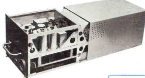
A pre-set frequency I.F. unit complete with 10 valves and power unit in wooden transit case, new and unused. Chock-full of components. Part of the transmitter receiver TR1366.
