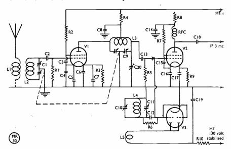
Fig. 2. The 58 mc converter circuit.
