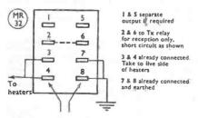
Flg. 2. Connections to the 8-way plug board at the rear of the BC-348 chassis. A 6 3 volt AC supply should be brought in as shown. Though the receiver can be muted by throwing the AVC switch to "off," HT is not cut; for this purpose a send-receive switch or relay should be wired across tags 2 and 6 above.
