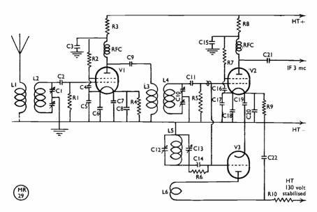
Fig. 1. Circuit of the 28 mc unit, as described in the text by G2IQ.
