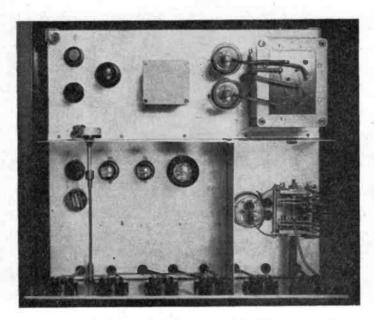
A top view of the G4NT rig, RF driver stage on lower left, with the 829 PA on the right. The modulator assembly is to the rear behind the vertical screen and uses 6537-635-616-P/P 807's in Class-AB1.
