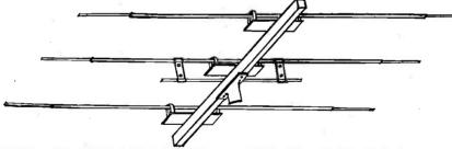
DURALUMIN ADJUSTABLE ELEMENTS, 9 ft. DURALUMIN BOOM, CAST ALUMIN HEAD, ADJUSTABLE "TEE-MATCH," SOLID COPPER FITTINGS.
