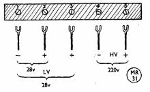
Fig. 1. The power supply tag-board as fitted to the BC-348 chassis. All spade ends should be disconnected before removing the dynamotor. The HV leads can then be taken to an external power pack. LT is obtained as shown in Fig. 2.
