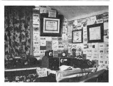
G2VV, Hampton-on-Thames, in 1934. The Tx was TPTG, with a 68-ft, end-fed aerial, and 25 watts into a Mullard TZO5-20. The Rx was 0-V-1.
