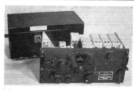
The BC-348 withdrawn from its cabinet. The space at the left rear on the chassis originally accommodates the dynamotor, leaving room for a mains power pack if desired. The inspection cover on the front panel exposes the underside of the valves in RF and FC positions.
