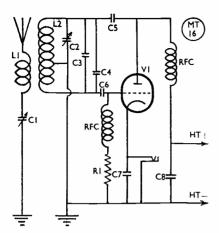
Circuit of the Hartley transmitter. A high degree of frequency stability is obtained by close attention to the details discussed in the text.
