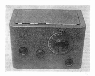
The 28 mc unit ready for work. Small-knob controls are for RF, mixer and band-set, with the large dial for band-spreading.
