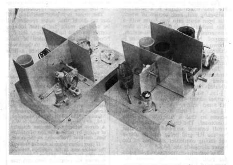
The 58 mc converter on the left, with the 6AK5 mixer compartment visible. The 28 mc unit is to the right, with the oscillator section nearest camera.
