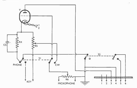
Fig. 4. Wiring of the control unit (Rx end). Terminations 1-2 are heater for V, 3-4 control line, 5-6 Rx HT S1 is a double-pole double-throw switch, shown in the "'Phone" position; S2, also DPDT, is at "transmit."
