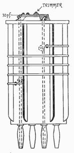
Fig. 3. BRS-7605's idea in diagrammatic form. The supporting wires are 16 SWG.
