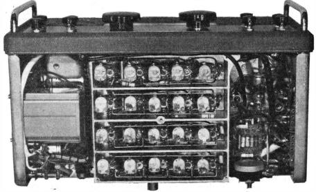
In the sub-space, showing the assembly of the tuning unit, which is built into a cast aluminium chassis
