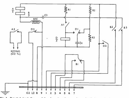
Fig. 3. Detached circuit diagram of the relay unit at the transmitter end. Black arrow heads A1, B2, etc., indicate that contact is made at these points when the appropriate relay is energised. Similarly, white arrow-neads at B1, D1 and D3 show that contact is broken, or change-over action takes place, when relays B and D are energised. Terminations 1-7 correspond to the circuit diagram on p. 304, July; 8-9 are for connection of the control-line pair; C2-L2 are connected as shown in Fig. 1.
