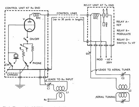
Fig. 1. The essentials of G4HM's system for CW/'Phone remote control, using only a single-pair control line. This line provides not only for remote actuation of the necessary relays, but also carries the audio input to the modulator, the keying impulses and the Rx aerial lead, all controlled from the receiver end. Such an arrangement allows complete freedom in the selection of an operating position.
