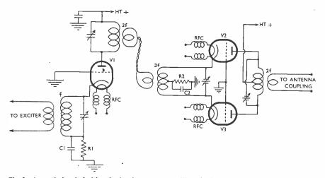
Fig. 2. A practical cathode-drive circuit using two stages. V1 is the doub er- say, from 29 to 58 mc-and V2,V3, comprise a push-pull amplifier, using TZ05-20's or a single DET-19. R1, R2 are the self-bias resistors and C1, C2, the bias resistor by-pass condensors.
