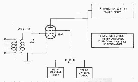
Fig. 3. Block layout of a single-side-band receiver. The highly selective tuning meter amplifier resonates at 50 kc and permits the selection of one side-band and carrier only. The 50 kc 2nd IF passes only the IF carrier plus about 4 kc of one side-band. This is selected by using one or other of the two crystal oscillators on 505 or 405 kc to generate the 50 kc IF.
