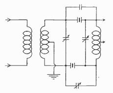
Fig. 1. Schematic of band-pass arrangement using two crystals. This is a standard circuit
