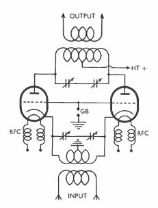
Fg. 1. Basic circuit for cathode drive RF amplifier
