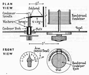
Fig. 4. The left hand contro sweeps an arm, carrying a meta cross piece, through the field of the main or band spread tuning condenser. By choosing dimensions correctly, the effect—somewhat similar to permeability tuning—can be made such that the signal on tune appears to be shifted slightly in frequency
