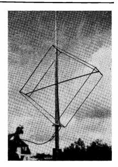
G2MV's square-beam aerial, lowered for inspection. The elements between the cross-pieces are \(\frac{1}{2}\)-wave for the frequency, and maximum directivity is broadside to the array.
