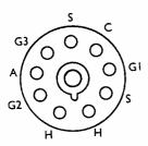
Fig. 1. Base connections of the EF-50. H, H, heater, C cathode, G1 control grid, G2 screen grid, G3 suppressor grid, A anode, S valve screen.
