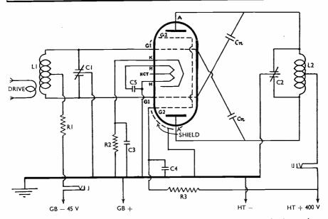
Fig. 1. Circuit around the QVO4-20, connected in push-pull. The neutralising wires in the photograph are represented by Cn. The electrodes are marked for reference to the valve base connection diagram, given at Fig. 2. Suitable RF chokes in series with the grid and plate coil centre-taps might improve balance. Heaters can be connected either in series (12-6 volts) or parallel (6-3 volts).
