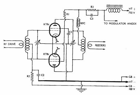
Fig. 2. Plate-and-screen modulation of a pair of tetrodes (KT8c's or 807's) in Class-C push-pull. Under the circuit conditions given, they will require about 10 mA drive. Values are: R1, 30,000 ohms, 3 watt; R2, 25,000 ohms, 2 watt; R3, 1,000 ohms, 40 watt; C1, ·001 μF, 600-volt DC working; C2, ·002 μF, 250-volt DC working; C3, 8 μF, 250-volt DC working.
