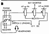
(A) is the wiring of the CW switch, (B) is for the Telephony change-over. Though four relays are shown, the operations in (A) and (B) could be performed by two relays only: One having three pairs of contacts (1, 3, 4, in B) and the other two pairs (1, 2, in A).
