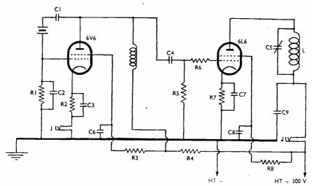
Fig. 2. The same circuit adpted for the use of the commoner 6V6 and 6L6 types in the CO and PA positions.
