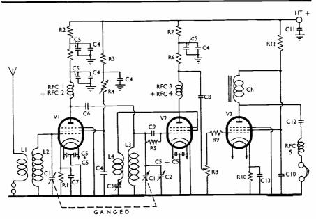
Fig. 2. Circuit of G5UM's straight receiver, fully discussed in the text. The use of the high-gain EF-50's, in a standard circuit with some refinements, ensures much improved performance over a similar receiver using ordinary valves. The form of construction adopted i a matter of taste, but a metal chassis and cabinet are desirable. Note that all components having the same values are numbered similarly.
