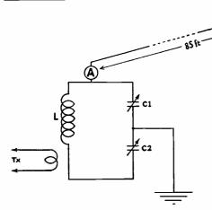
The Matched End-On aerial coupler. C1, C2, should be .0005  $\mu$ F for all-band operation 1.8-28 mc, or .0002  $\mu$ F for 7 mc upwards. The system will also take power very effectively on 58 mc with smaller condensers and careful adjustment. Coil details are given in the text. A is an aerial ammeter, either hot-wire or thermo-couple; a 5- or 6-volt bulb taking about 1 amp. will do i a meter is not available.
