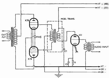
Fig. 1. A Class-B modulator. It will give sufficient output to control a 100-watt carrier. In this circuit, C1 can be 4 µF, C2 8 µF, and R 1,000 ohms. The screen connection should be made by strapping them together, by-passing to earth with a 8µF 400-volt DC working condenser, and feeding through a 2000-ohm 10-watt resistor connected to the HT positive line.
