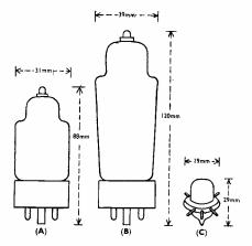
Fig. 2. Comparisons in valve types. (A) is an RF pentode specially designed for shortwave use; (B) is a corresponding valve for medium waves; (C) is an acorn-type triode designed for use on ultra-short waves—say, below 5 metres (60 mc).
