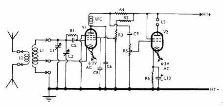
Fig. 4. A two-valve mains-operated receiver, with electron-coupled reaction circuit and band-spread tuning. The circuit of a mains power unit for this receiver is given in Fig. 5.
