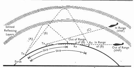
Fig. 1. Showing the propagation of radio waves at different frequencies.
