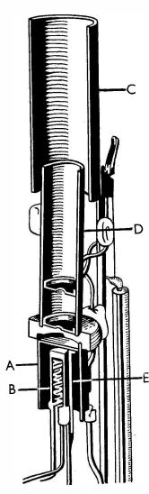
A—Grid. B—Heater. C—Anode 2 D—Anode 1. E—Cathode.
