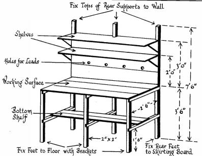
Length of Working Surface 6ft · Width of Working Surface 2ft 6ins
