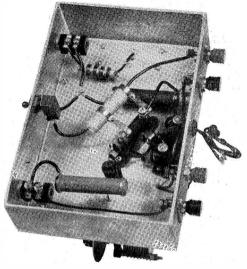
Underneath the CO unit. The 6 BA screws holding the upperside components are used to secure the condensers in the sub-space.
