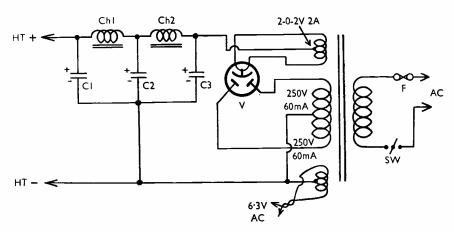
Fig. 5. A mains-operated power unit for the operation of a receiver such as that shown in Fig. 4.
