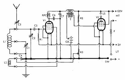
Fig. 3. Circuit of an excellent two-valve battery-operated receiver suitable for operation on wavelengths between 10 and 100 metres (30 and 3 mc).
