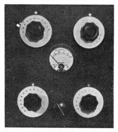
The compact 56 Mc CC CW/'Phone transmitter built by A. W. Fawcett, G2HQ, Sheffield. Though four valves are used, the panel is less than 9-ins. square.
