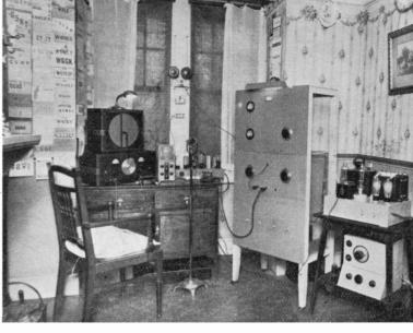
tioned pushes a pair of zero-bias 203Z's in a Class-B unit, giving about 300 watts of audio.
