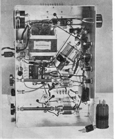
In the sub-space of the "Two-Band Two," showing lay-out of parts and general arrangement of wiring. Note the flex ble coupler controlling the grid-excitation condenser C6. The coil and condenser in the foreground are for ECO operation.
