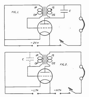
sufficient for 'phones. It is best to try all the battery triodes available, to see which gives the best note, while the LF transformer can be the odd one to be found in every junk box. The pitch of the note can be varied by trying different condensers at C, or across IP and OP, as shown dotted.
