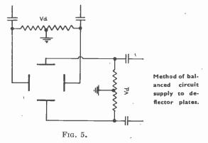
In order to overcome both of these forms of distortion, the plates should be connected in symmetrical push-pull arrangement as shown in Fig. 5 in which both plates of a pair are connected to the anode through an impedance of equal value, and oscillate in potential symmetrically about the earth potential of the anode.
