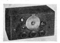
Complete coverage from 12-2,000 metres in 5 bands. Separate Bandspread Condenser, Beat Frequency Oscillator. Phone Jack. Send-Receive switch. Aerial Trimmer. Provision for single-wire or Di-pole International Octal Valves. For 200-250 v.
