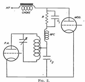
Fundamental circuit for choke control modulation. The choke should be 15 henry, and capable of carrying the plate current for both PA and modulator valves. Cl is 2 mF, C2 is not more than '002 mF, while the value of R is best found by experiment as discussed in the text.
