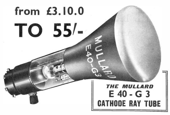
ERE is a great bargain for amateur transmitters—the Mullard E40-G3 Cathode Ray Tube at a reduction of 15/-. Invaluable for measuring modulation percentage, checking for distortion in amplifying equipment, observing the effect of circuit alterations and for general experimental use. The tube is of the high vacuum type, with a 3 inch screen, employing double electric
