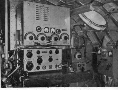
being ganged to one dial. CW, ICW and telephony can be received at will, and separate volume and reaction controls, with a two-way wave-band switch, are provided.
