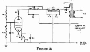
Fig. 2 shows a typical circuit. R1 and R2 are the screen potentiometers decoupled by C1. R3 and R4 are the cathode bias resistors decoupled by C5. Resistor R4 is to prevent the removal of all bias from the valve. L1, L2 and C2 are as in the pre-
