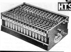
THE MILNES H.T. SUPPLY UNIT is a battery of alkaline cells with nickel-cadmium plates. It is fitted with an ingenious trouble-free switch whereby banks of four cells can be connected in parallel for automatically regulated charging from a 6 v. L.T. accumulator. With the switch in the opposite position, all cells are connected in series. siving H T. voltare. in series, giving H.T. voltage.
