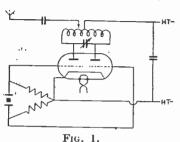
The centretap of the filament transformer should be connected to the negative H.T. This connection is not shewn in the circuit because most amateurs connect this as
