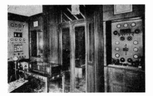
Remote control of all transmitters is possible from the operating table of G5BY. Left to right; 500 watt modulator, transmitter remote control board, receivers, 250 watt 3.5, 7, and 14mc transmitter. Note the first British W.A.C phone certificate and the trophy for the 1929 A.R.R.L. award for the world's best amateur station.
