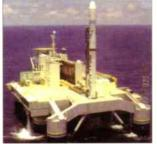
Aerial view of the 'Sea Launch' rocket platform, a modified oil drilling rig. Control operations are from a nearby ship.
