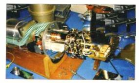
A receiver cryostat under construction. This is one of fourteen 33GHz receivers which will form part of the Very Small Array (VSA) on Tenerife to study the radiation originating in the Big Bang.
