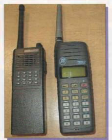
Two popular MPT1327 trunked radios. The radio on the left is a Kenwood TK-255 while the one on the right is a Tait T3000. The Tait's large display lets its users receive text messages just like a mobile phone.
