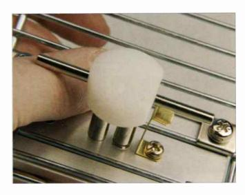
The radiator with the tuning strip fitted for optimum amateur performance.
