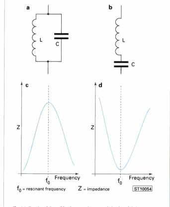
Fig. 6.1: Two L and C combinations creating a tuned circuit and their response curves. See text for more detail.
