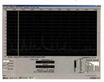
The plot of the loop in action - MSF is the signal in the shaded portion.
