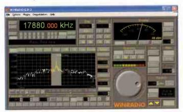
The receiver is extremely sensitive, making it possible to comfortably read CW signals well under -130 dBm input lea yet featuring a respectable 95 dB dynamic range ma receiver resistant to strong signal overload.
