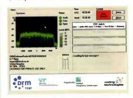
Fig. 2.3: Perfect reception from DW on 6.140MHz. Notice the shape of the DRM spectrum and that all status lights are green.
