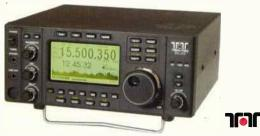
**RX350D** The Ten-Tec **RX-350D** is a full featured, mid-price range HF DSP receiver. Now even more versatile due to the **inclusion of the 12kHz I.F. socket on the rear panel for DRM use** (demodulation software required). On-screen band activity display adds a new dimension to locating transmissions
