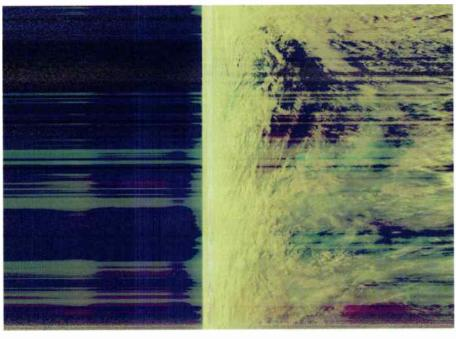
Fig. 1: FY-1C 1628 11 September showing unsynchronised scan.
