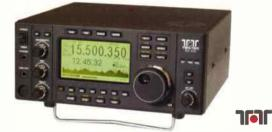
**RX350D** The Ten-Tec **RX-350D** is a full featured, mid-price range HF DSP receiver. Now even more versatile due to the **inclusion of the 12kHz I.F. socket on the rear panel for DRM use** (demodulation software required). On-screen band activity display adds a new dimension to locating transmissions and tuning the receiver, 34 DSP bandwidths provided, noise reduction etc. *£999.00 inc VAT, UK carriage £10.00*
