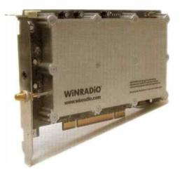
The high sensitivity is also matched by that of the S-meter: The calibrated S-meter shows the received signal levels in dBm,  $\mu$ V or S-units, down to the receiver noise floor. The IF bandwidth of the receiver is continuously adjustable from 1 Hz to 15 kHz, in 1 Hz steps.
