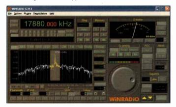
The receiver is extremely sensitive, making it possible to comfortably read CW signals well under -130 dBm input levels, yet featuring a respectable 95 dB dynamic range making the receiver resistant to strong signal overload.
