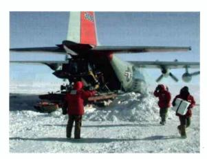
Byrd Field Camp workers prepare to unload a Challenger tractor from the rear of an LC-130 aircraft. Photograph - Mark Sabbatini. Courtesy NSF 2004.
