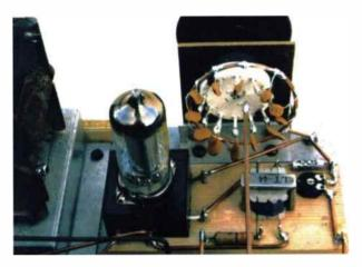
• Fig. 11: The switched capacitor r.f. tuning assembly.
