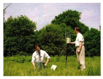
• Some claim that radio-noise levels are already so high that the effect of new sources is insignificant. The BBC has made various measurements to refute this argument. This photo shows BBC engineers measuring radio noise in the short wave bands in a typical suburban garden at a quiet remote site for reference.
