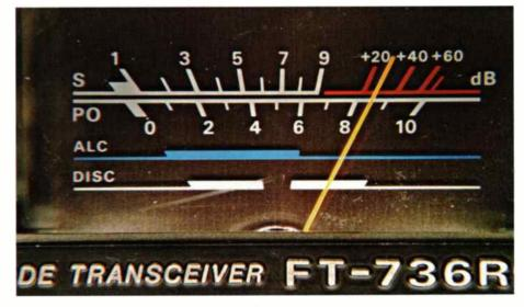
particular 'law'. This doesn't matter because the 'S' meter can be scaled to indicate correctly, but unfortunately, it seems that many manufacturers don't seem to do this. Perhaps they think it is more aesthetically pleasing to have the meter scale graduations equally spaced.
