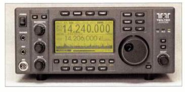
he Ten-Tec Jupiter 538 transceiver has just achieved CE/ETSI approval following several months of evaluation and testing. The first CE stock will be available in the UK from early July 2003. Output power is variable from 5-100W from 160-10m, s.s.b., c.w., f.m., The Jupiter 538 provides 34 DSP bandwidths on receive, general coverage, triple conversion and more.
