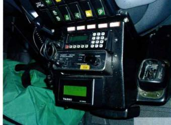
The rack stack in the ambulance, showing from the top: Yaesu VX-1000 MPT1327 set, then the VXR-2000 repeater set and finally at the base, the display unit.
