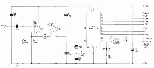
Fig. 3.12: NAVTEX Decoder circuit diagram.
