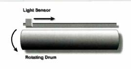
Basic principles of h.f. FAX operation. tracks the light to dark changes in the document. When this signal is applied to a radio transmitter, it is used to vary the carrier frequency of the transmission.
