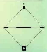
The loop is constructed of flexible twin cable braced by a centre pole
