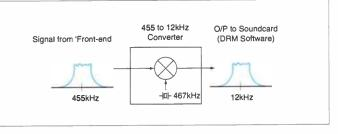
Fig. 2: The block diagram of a converter to produce baseband output from a 455kHz i.f.
