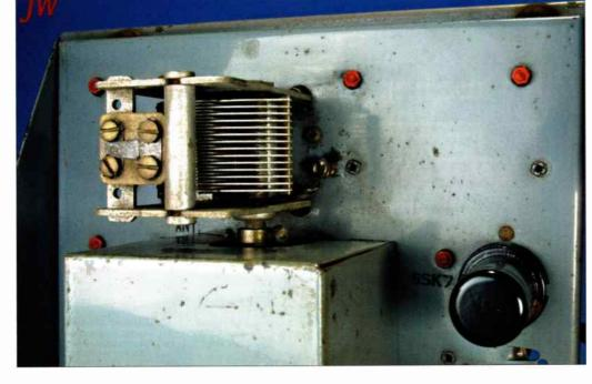
R-50M the separate r.f. stage variable capacitor.
