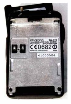
The two screws at the TH-F7E Step 2 bottom need removing too.
