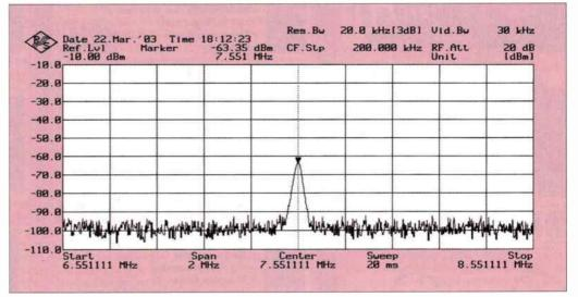
Fig. 3: For reference, the BC348 local oscillator output measured at the antenna socket.
