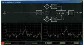
The Professional Demodulator (optional) Includes Interactive block alagrams for all modes, with two real-time spectrum scopes and THD and SINAD measuring facilities.
