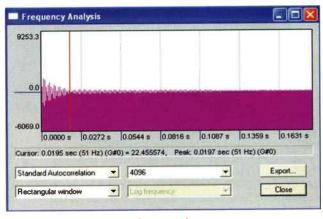
Baud rate detection using Autocorrelate.
