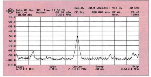
Fig. 2: R-50M local oscillator output measured at the antenna socket. Significantly less that the TCS-12.
