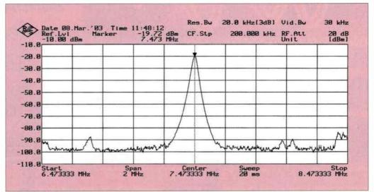
Fig. 1: TCS-12 local oscillator output measured at the antenna socket, an amazing -20dBm.
