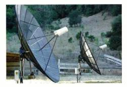
SETI Institute's Rapid Prototype Array taken in August, 2000. The RPA was built near the University of California's Berkeley Leuchner Observatory to test engineering concepts for the planned Paul Allen Telescope.
