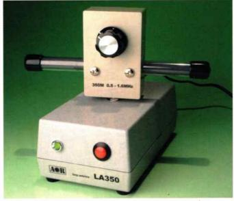
The element simply plugs into the base unit. Pictured is the medium wave bar.
