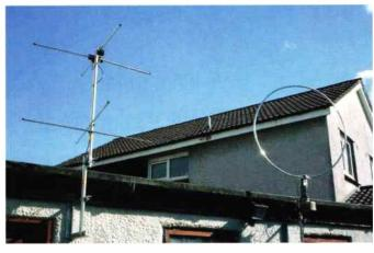
Here are Dougie's two external antennas: a turnstile for satellite work and a Wellbrook ALA1530 active antenna for h.f. There is also a long wire and a host of internal antennas mounted in the loft.
