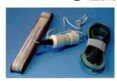
Graham Tanner's Revco Angler portable short wave antenna. The 45m roll of antenna wire is to the left, and plugs into the balun (top right). From the balun, the signal solits to either the **BNC** connector (black lead) or crocodile clip (green lead).
