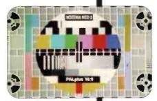
Fig. 3: The Dutch modified PM5544 test card with wide-screen 16:9 aspect ratio.
