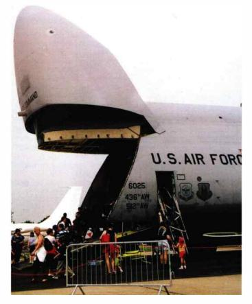
Lockhead C-5B Galaxy at the RAF Mildenhall Air Fete in 2001. The open nose allows out-sized loads to be easily moved in and out. The spectators in the foreground show the massive proportions of the aircraft. (Photo: Graham Tanner).
