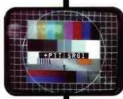
Fig. 3: The FuBK test card radiated in the Seventies by the Swiss +PTT.
