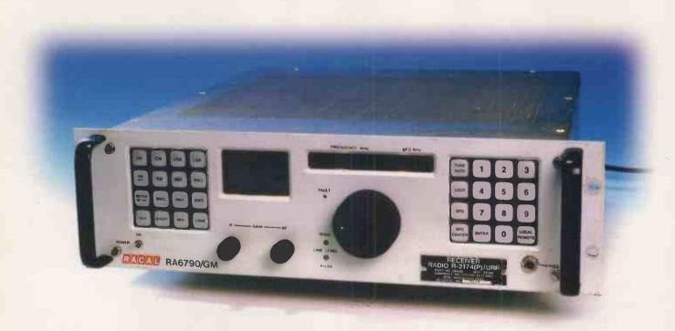
weighted for the right 'feel' and placed at just the right height above the bench top for comfortable operation. Above the tuning knob is a long l.c.d. which shows the operating frequency down to 1Hz, with a sub display showing b.f.o. offset to ±8kHz in steps of 10Hz. The b.f.o. display is only shown when in c.w. mode.
