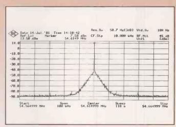
Fig. 4.The RA6790's first conversion oscillator plot, not as good as a RA1792!
