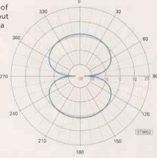
Fig. 2: Figure-8 dipole horizontal pattern.
