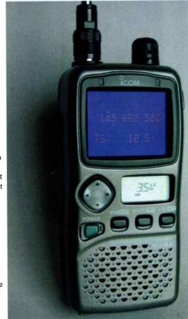
memory channel, bank and mode indications and a bargraph S-meter to give you an idea of the relative signal strength of the transmission you're listening to. But if that's not enough, you can also bring the larger colour LCD into use to give you a larger and more colourful text display of the frequency, mode, and so on.
