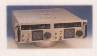
Johnson HF-1000, it was inevitable that I would also take a look at the Cubic 3030A. The test set-up, in case you missed the original description, was to put the receiver on a wooden table, 800mm above a ground plane in an r.f. anechoic chamber, and with an active whip antenna as used in military emissions testing placed at a distance of 4m from the receiver front panel.
