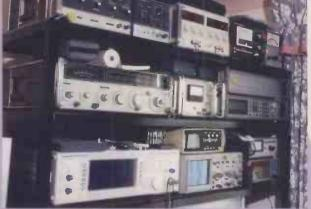
A substantial radio test set-up consisting of HP 8620 Sweep Oscillator, Escort ECG-3230 Sweep Function Generator, Marconi Audio Power Meter 893B, HP RMS Voltmeter 3400A, HP 8640A Signal Generator, Racal Instruments Rubidium Frequency Standard 9475, Racal Dana 9478 Frequency Display Unit, Marconi Instruments 2030 10kHz to 1.35GHz Signal Generator, Tektronics 2232 100MHz Digital Storage Oscilloscope, Farnell True RMS Sampling RF Voltmeter TM8 and Racal Dana 1992 Universal Counter.
