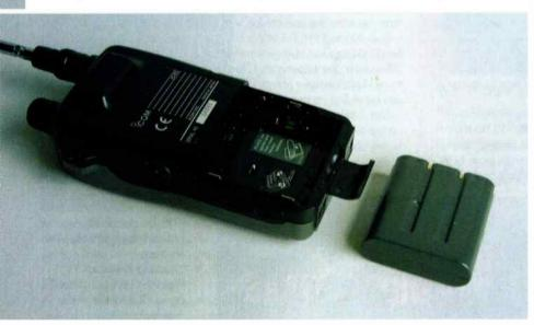
AM Broadcast: 0.495-1.620MHz HF: 1.625-29.995MHz 50MHz: 30.0-75.995MHz FM Broadcast: 76.0-107.995MHz VHF Aircraft: 108.0-135.995MHz 144MHz: 136.0-255.095MHz 300MHz: 255.1-382.095MHz 400MHz: 382.1-769.795MHz 800MHz: 769.8-960.095MHz 1200MHz: 960.1-1399.995MHz
