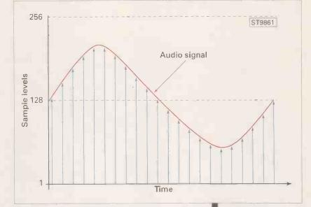
the input signal at regular intervals. The results of these measurements are then stored as a number ready for the computer to process.
