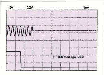
Fig. 3: The trailing edge of the burst shows the audio carrying on after the r.f. input signal has stopped.
