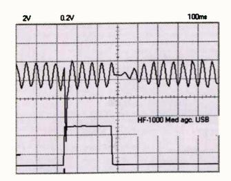
Fig. 2: The detail of the leading edge of the r.f. step with the audio containing an uncontrolled oscillation, which starts about 5ms after the incoming r.f. signal.
