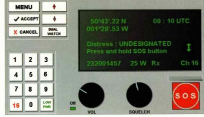
Fig. 2: DSC controller sending distress message.
