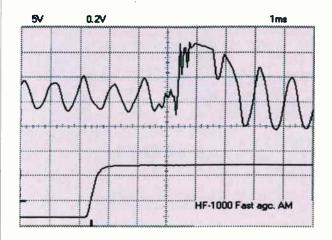
Fig. 4: The leading edge of audio in a.m. mode generating the same uncontrolled 'pop'.
