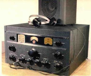
Selectivity in the AR88D is provided by having three i.f. amplifier stages embracing a total of twelve tuned circuits at 455kHz (735kHz in the AR88LF) and a single crystal filter. The crystal filter is not tunable from the front panel as in the case of receivers like the HRO, so keen c.w. operators would miss the 'single signal' razor sharp peaks and notches, but the design and alignment of the crystal filter is such that the resultant bandwidth is more or less symmetrical.
