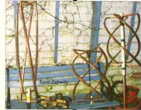
Fig. 6: Comparison QFH antennas under test by Paul Hayes.
