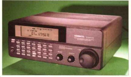
a  $50\Omega$  BNC external antenna input, a 3.5mm external speaker socket, and sockets labelled 'Tape Out' and 'Tape Remote'. This last socket allows you to connect a tape recorder with an external pause control facility to the COM225 and have it start automatically recording when one of ten user-selectable memory channels is selected. I'd have liked to be able to use this facility with more than just ten out of the 500 channels, but at least it is there.
