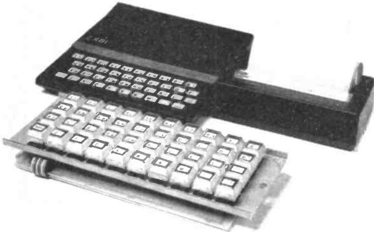
**A vast improvement over the standard keyboard featuring a unique two PCB construction.**
