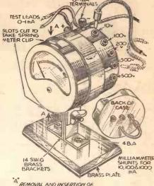
A REMOVAL AND INSERTION OF METER REQUIRES SLIGHT PRESSURE ON CLIP ENDS TO CLEAR SLOTS.
