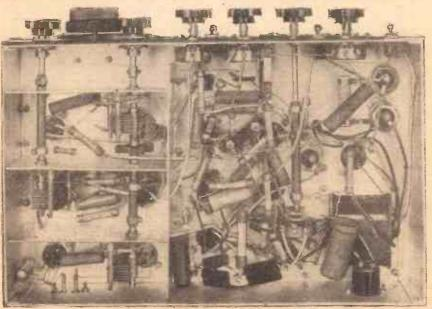
Underside of chassis, showing the band-setters and method of screening.
