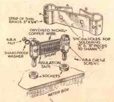
A neat method of arranging a meter shunt.
