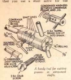
cutter. For the shank I used an old disctype condenser scale bush, and this being of brass, it proved easy for drilling and tapping. From the illustration it will be noticed how a comparatively fine adjustment can be obtained by providing the tapped holes at carefully located centres so that a fractional difference results in stepping the grub screw up or down.
