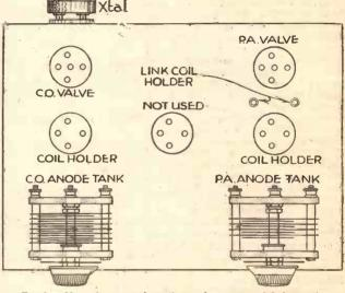
Fig. 2.—How the original oscillator chassis is modified to allow the P.A. stage to be added.
