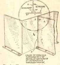
Fig. 4 .- Illustrating one of the causes of crackle between screens.
