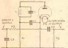
Fig. 2.—A.C. and D.C. components are shown here and suggested values are :— $R_1=0.5$  meg.;  $R_2=2$  meg.;  $R_3=1$  meg.;  $C_1=.0001$  mfd.;  $C_2=.01$  mfd.;  $C_3=.05$  mfd.
