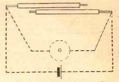
Fig. 1.—Two parallel wires form a small con-denser, which can be charged and discharged.
