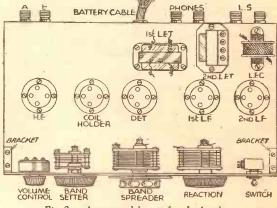
Fig. 2.- A suggested layout for the 4-valver.
