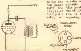
Fig. 3 (left). The S.G. value may be parallel-fed as shown. Fig. 4 (right). Connections to the valve-holder of the S.G. valve.
