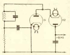
Fig. 5.—A signal limiter built round two diodes.
