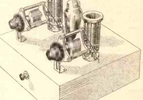
Fig. 3.—A suggested experimental chassis (10in.×10in.×3in.)
