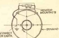
the earthed brush is recognised it is a simple matter to remove the brush holder and insert some insulating washers underneath to insulate the whole from carth on the
