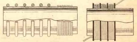
Fig. 3.—Self-capacity of a coil can be reduced by increasing the spacing of the turns, using finer gauge wire or, in the case of a pile winding, by dividing the winding into a number of sections.
