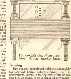
for several hours before ironing up. convenient, leave it to dry overnight before the fire, or stand it on a sheet of newspaper over the hot-water storage tank. The former illustrated will require approximately 90 pairs of .014in. stampings,
