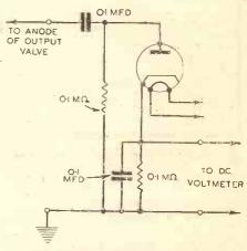
Fig 7 .- A successful output meter rectifier using a diode valve.
