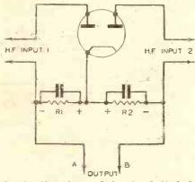
Fig. 6.-Here the two diodes of a double-diode value are used separately on two H.F. inputs.
