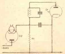
Fig. 4.—In this circuit two diodes are used—one for the signal rectification and one for bias.
