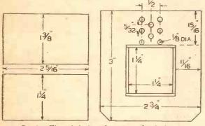
Fig. 1.- The end checks and core strips for the former.
