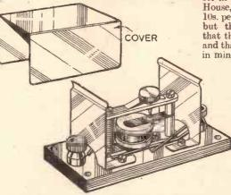
Fig. 4.—Showing the constructional details of a good highnote buzzer.
