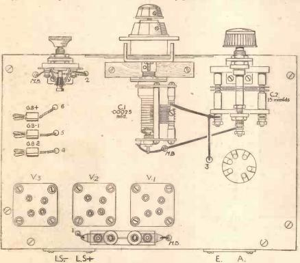
Top chassis view of the Prefect S.W. Three showing the band-spread tuning combination.
