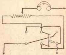
Fig. 4.—A change-over switch may be used with the potentiometer as shown here.
