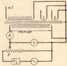
Fig. 1.—Break-down test. Voltage regulator R is adjusted till at least twice the working pressure is applied to the primary winding. O/L is an overload release.
