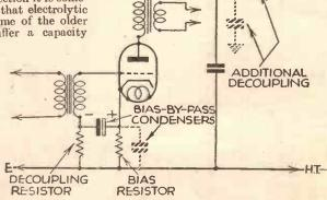
Fig. 2.—Grid and anode circuit decoupling, which should be checked.
