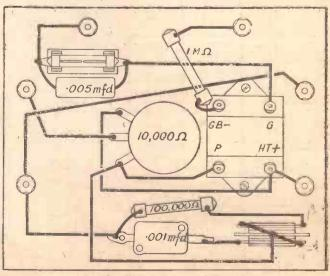
Fig. 5 .- Wiring diagram of the meter.
