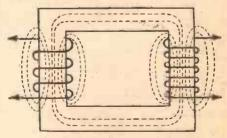
Fig. 3.—Diagram illustrating leakage flux.
