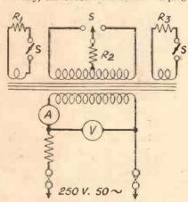
Fig. 2.—"Overall" test for regulation, output and efficiency.
