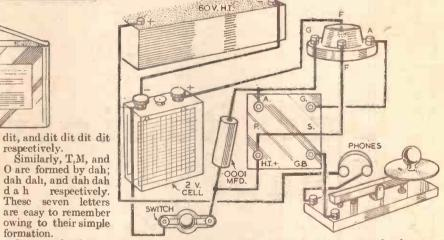
letters Fig. 2.—The method of connecting an L.F. transformer and valve as an posites;
