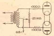
Fig. 4.—Stability of a push-pull circuit might sometimes be improved by using the connections indicated.
