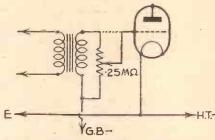
Fig. 5.—Method of obtaining stability and L.F. volume control at the same time by using a .25 megohm potentiometer.
