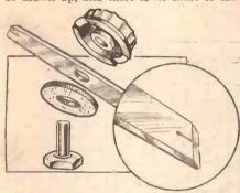
Fig. 3.—How the pointer is made and assembled.
