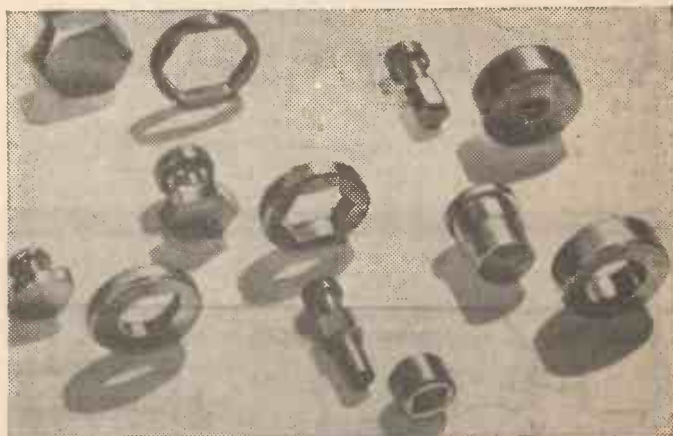
1 A variety of parts showing the varied shapes which can be produced directly on a lathe fitted with a polygon tool box.
