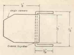
Fig. 2.-Details of tape retainer.
