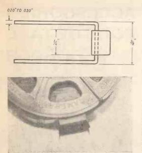
Fig. 3.- The tape retainer fits into the spool.
