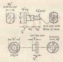
Details of the pivot bolt and pivot bush.
