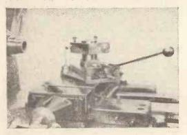
Setting the cutter point to centre height with the aid of the gauge pin.
