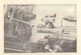
Setting the tool pivot point to come under the centre of the ball blank.
