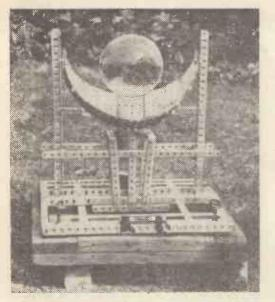
METEOROLOGICAL Office pattern sunshine-recorder is an expensive instrument, and amateur observers may be interested to hear of a cheap and acceptably accurate instrument which I have made for my own use. This article was first published in "Weather", November 1962 and is reprinted by their permission. It will be seen that the construction of this instrument entails little cost and no special skill.
