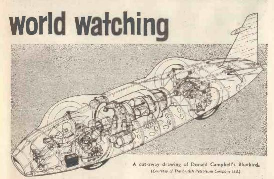
new tyres into use. This has the advantage that it avoids the necessity of inspections for accidental damage and in any case the tyres themselves will be too hot to handle immediately after a run. The turning circle of the car is 300ft, equivalent to a lock of only 5 degrees each way.
