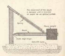
Fig. 3.-Simplified diagram of a Seismograph.
