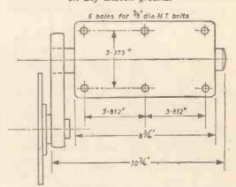
Plan view of a Flexitor unit without wheel. Attach to cross members with G-cramps so that the wheel "toes in " correctly then drill fixing holes to suit. Toe in from wheel rim to trailer centre line should be  $\frac{1}{16}$  in. for 8-10 in. wheels,  $\frac{3}{12}$  in. for 12-13 in. wheels and  $\frac{1}{6}$  in. for 16 in. wheels.
