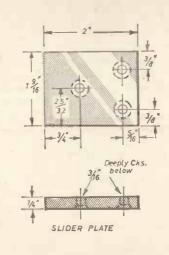
Top left.—The completed ball turning tool. Left.—The base and slider plate constructional details. Below right.—The gib strips. Below left.—The tool set-up during a ball turning operation.
