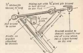
To operate the trailer leg mechanism the screw is turned with a wheel brace. The moving nut thus travels along the screw and the leg is raised or lowered. With such a leg at each corner it is possible to support the trailer firmly in a level position on any uneven ground.
