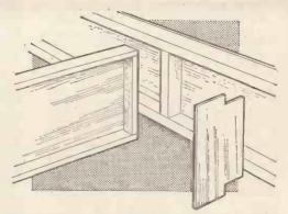
Fig. 7.-Fitting the tailplane ribs and extra gussets to the tailplane rear spar.
