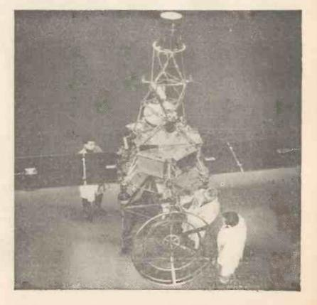
plete a checkout of a Mariner spacecraft prior to installing it on an Atlas - Agena B rocket. The 447lb package contains instruments to measure the temperatures on Venus and study magnetic fields and charged particles in interplanetary space.
