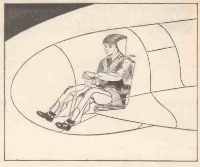
Artist's drawing shows how inflated bladders and netting are used in a new restraint system to prevent space pilots from making injurious movements during emergency escape.
