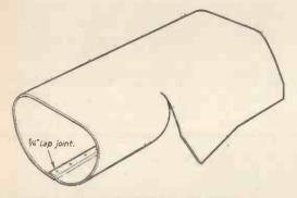
FIREBOX AND COMBUSTION CHAMBER AFTER BENDING. Fig. 126.
