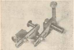
Mandrel dividing attachment with bracket added for compound dividing.
