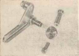
Dividing attachment bracket for compound dividing, with modified drawbolt.
