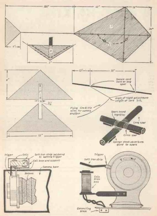
the small piece of metal that holds them together on the metal frame, and the armature. The camera to be used for the aerial photograph governs the position in which the tripping unit should be mounted. In the writer's prototype, the camera used was an old "Coronet" that had seen many good sights at ground level, and was considered by modern standards as being "out of date".
