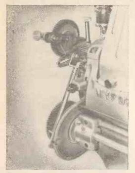
Compound dividing attachment set up for 24 divisions; 40t wheel on mandrel, meshing with 20t wheel keyed to 60t indexing wheel.
