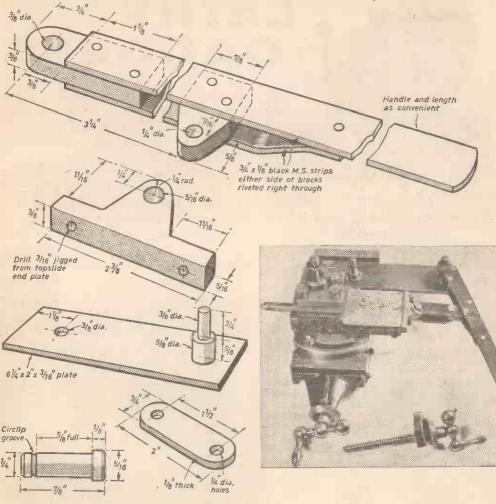
for the hole in the base plate. Countersink the hole in the plate underneath and rivet the pin tightly in position, filing down flush after riveting.
