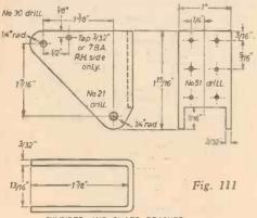
CYLINDER AND SHAFT BRACKET.
