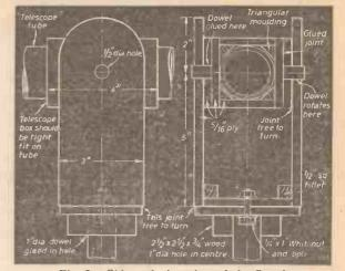
Fig. 3.-Side and plan view of the Stand.
