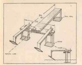
This highly simplified model can be built in a few hours and when towed at some 8-10 m.p.h. will demonstrate the remarkable stability and seaworthiness of an incidence control system. It will negotiate waves of 5tt high with ease.
